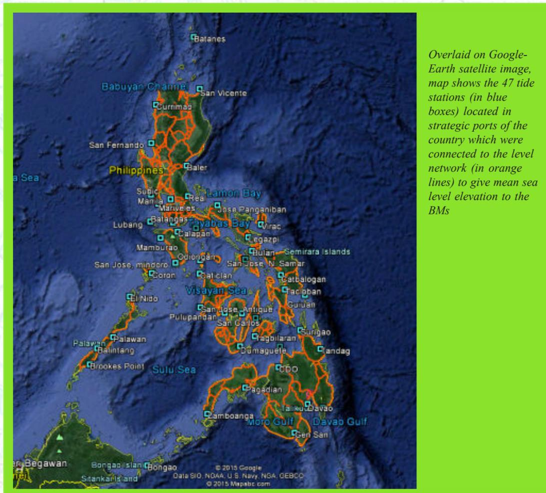
*Overlaid on Google-Earth satellite image, map shows the 47 tide stations (in blue boxes) located in strategic ports of the country which were connected to the level network (in orange lines) to give mean sea level elevation to the BMs*
