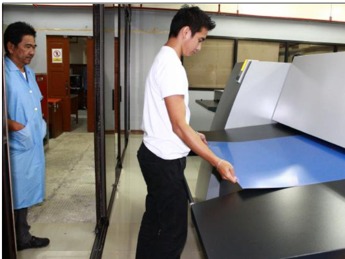
Inserting thermal plate for automatic plate exposure in the CTP machine
